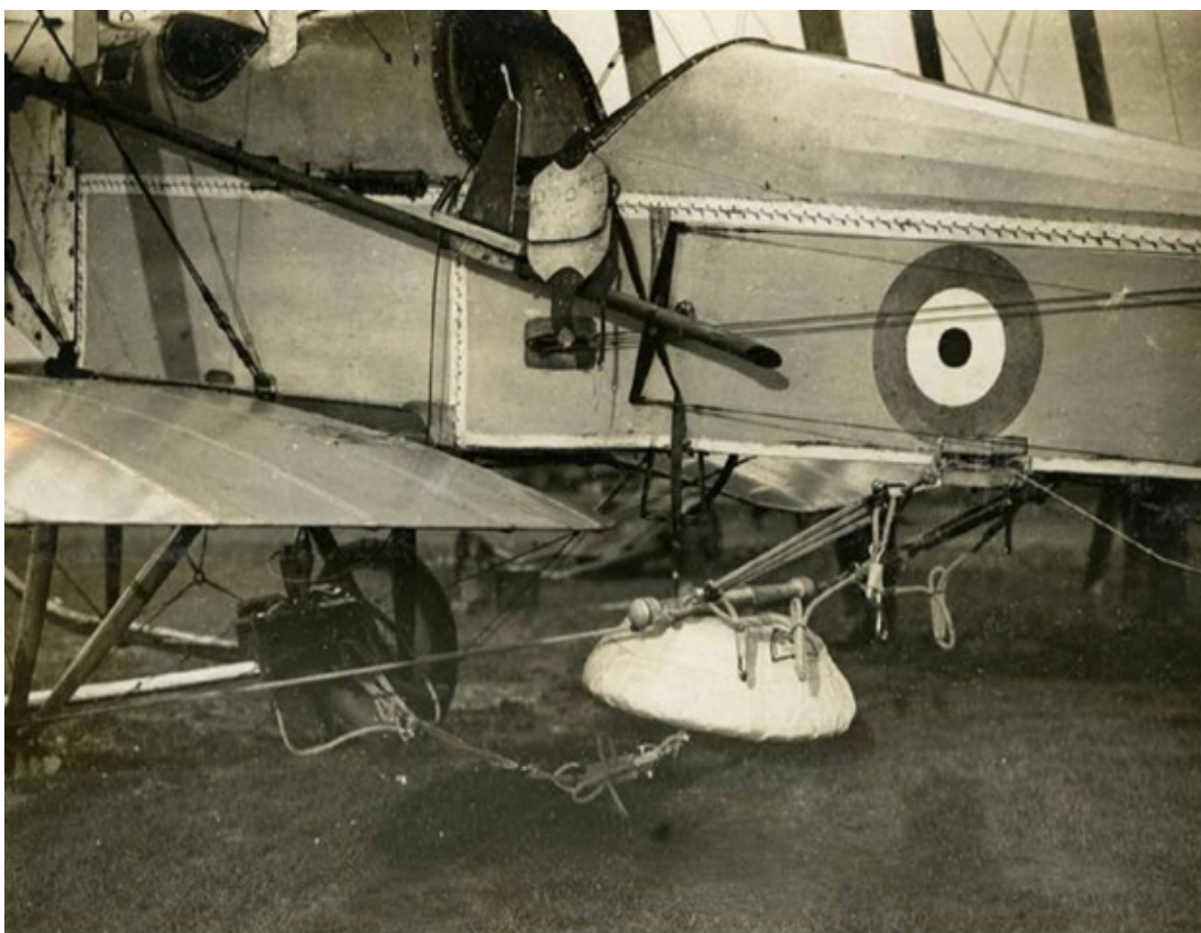
Photograph 5. Calthrop parachute installed under a BE-2c. Used with permission of Great War Aviation Society.
